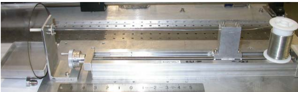
Figure 6. Proof-of-concept light metal wire propellant management system
